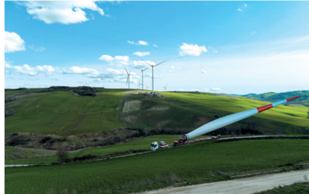
The blade lifter makes it possible to transport long rotor blades even on twisty roads.
